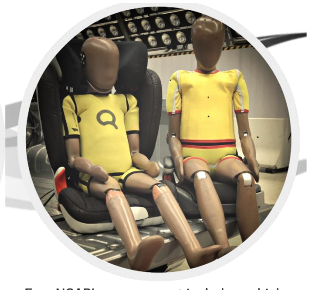
Euro NCAP's assessment includes vehicle provisions, CRS installation and Q6/Q10 testing
